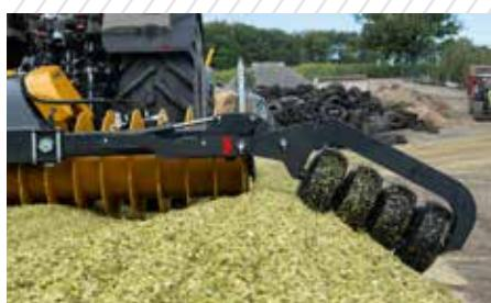
*For secure compaction in silos without walls, we recommend using an edge compactor.*
