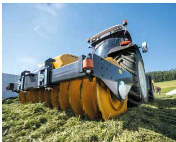
*When using the SILO KOMPAKT, a uniform compaction with a high depth effect is achieved across the entire working width.*
