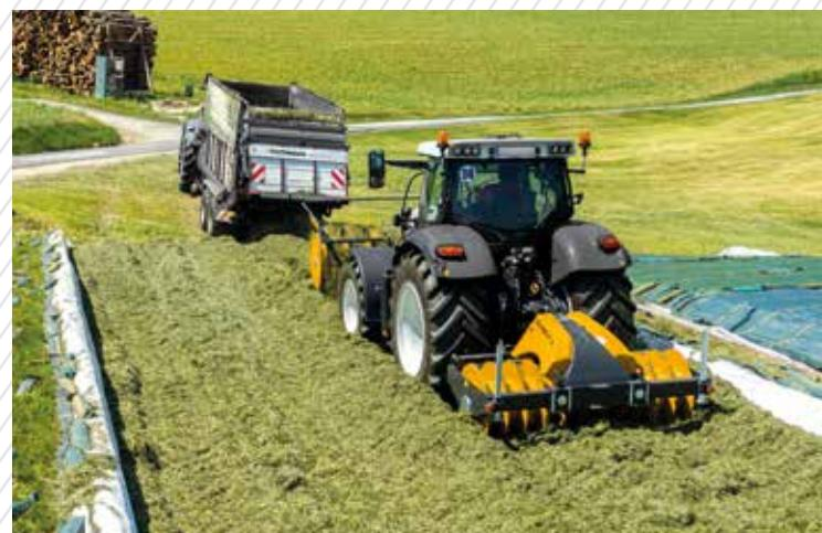
*Ensiling with the highest efficiency: With the combination of silage spreader and silage roller, the feed can be distributed and compacted in a single step.*
