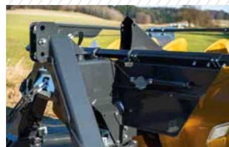
The baffle plate package (standard on the SF Koloss) ensures that the feed slides off quickly and prevents deposits on the unit.
