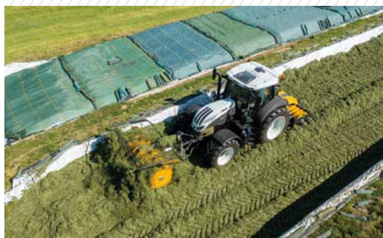
*Maximum efficiency: distribution and compaction in one work step.*
