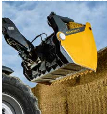
*The closed bottom of the cutting bucket is ideal for preventing feed losses during transport.*
