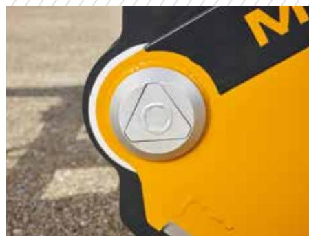
*The large main bearing pin (type N, M: 50 mm Ø / type H, XL: 60 mm Ø) guarantees a long service life for the silo cutting bucket.*
